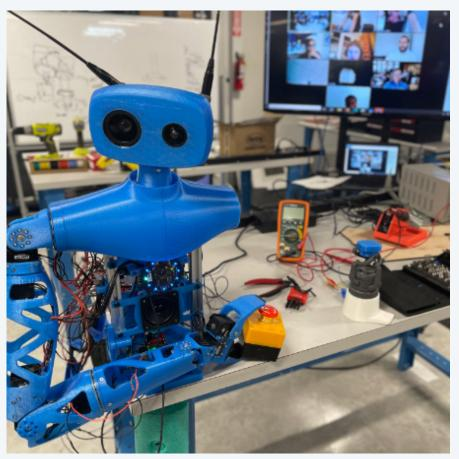
Reachy, an open source robot from Pollen Robotics, was built during one of the Mechlabs programs. In another program, incoming students at SJSU built DIY Robocars, trained the machine learning algorithms and had a car race.
