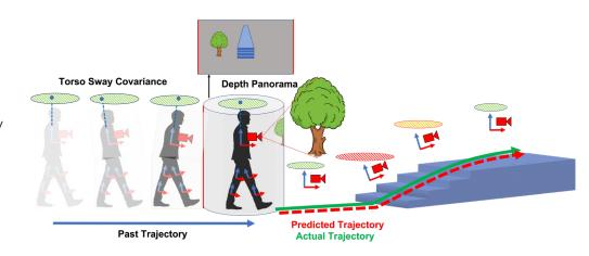
Picture 9: SmartBelt: Human Motion Prediction and Fall Prevention from Wearable Sensor. All images are courtesy of Stanford ARMLab
