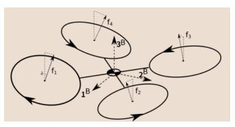
UAV with tilted propellers away from common thrust direction which helps improve total power consumption. All images are courtesy of UCB HiPeR Lab.
