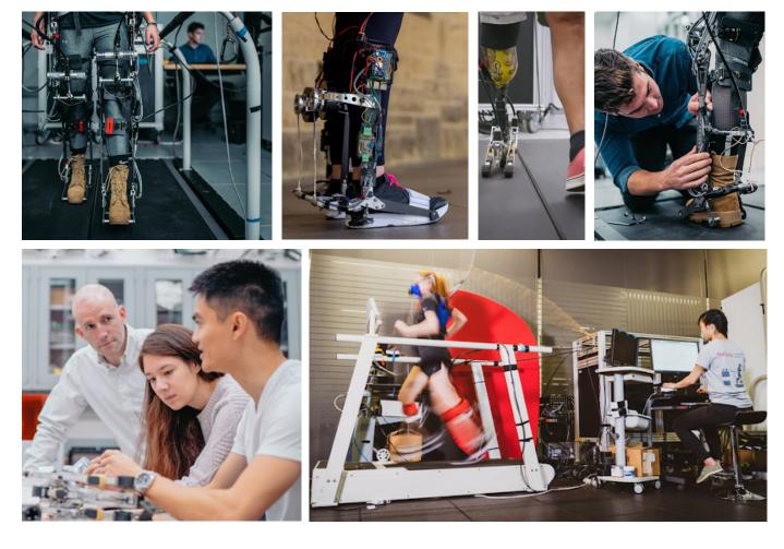
Prothesis and exoskeleton robots that help improve efficiency, speed, and balance. All images are courtesy of Stanford Biomechatronics Lab
