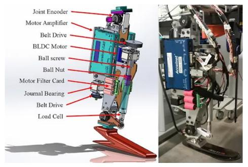
Design and Manufacturing of a Powered Knee-Ankle Prothesis All images are courtesy of SFSU CARE Lab
