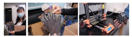
In tactile sensing and haptic control, we design, model and fabricate soft exoskeletons and wearable electronics. Among them is a wearable master-slave glove, which can communicate with haptic feedback wirelessly through ESP32. We are interested in using them for manipulation, teleoperation, and remote surgical training tasks.
